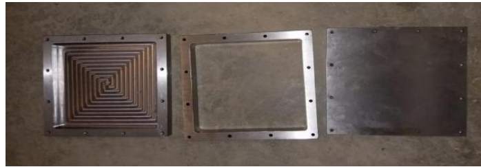
Figure 46: Parts after welding, drilling, and finishing
