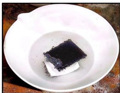
Figure 2: PV cell sample dipped in Benzene
