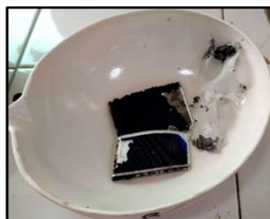
Figure 3: EVA removed from PV cell Sample
