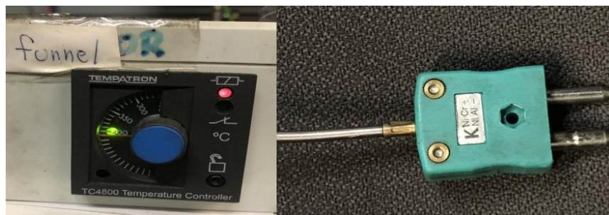
Figure 43: The PID controller and K-type thermocouple
